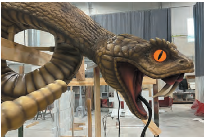
■ Hardcoat foam with structural supports and outdoor UL-rated lighting integrated.
